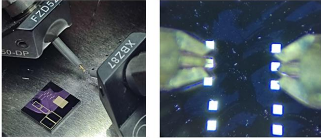
Fig. 13: (left) photo of the die under test on probe station and (right) microscope image of a HEMT device during RF characterization.
