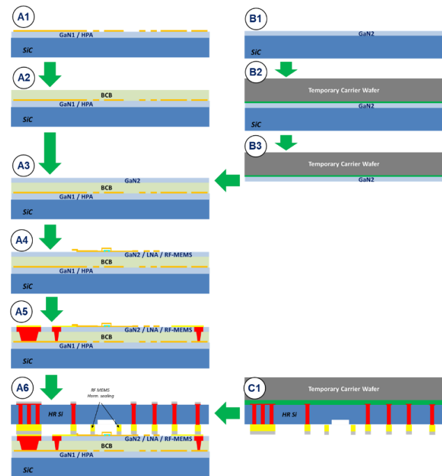
Fig. 1: schematic process flow for 3D sequential integration
